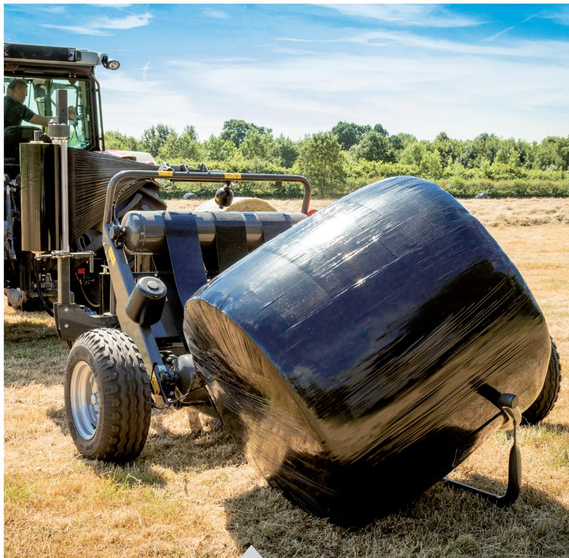
Bale discharge is exceptionally gentle, without the risk of damaging the film, thanks to a low-positioned wrapping table which tilts close to the ground when unloading bales. An optional baler tipper is available to prevent the bales from rolling in hilly conditions, improving safety and reducing the time required for bale collections in the field.
