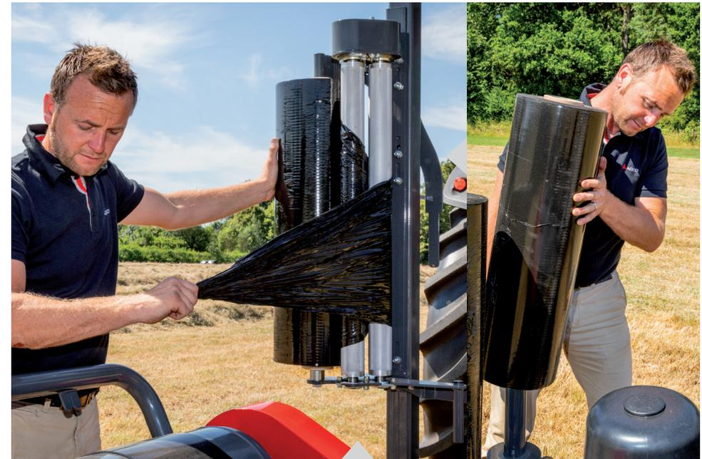
Depending on the crop and conditions, the operator can easily adjust the required number of film layers. The pre-stretching device is designed to work with 500mm or 750mm rolls and can be set at 55% or 70% stretch for tighter wrapping and reduced film consumption. A quick-lock system makes the replacement of empty rolls fast and easy.
