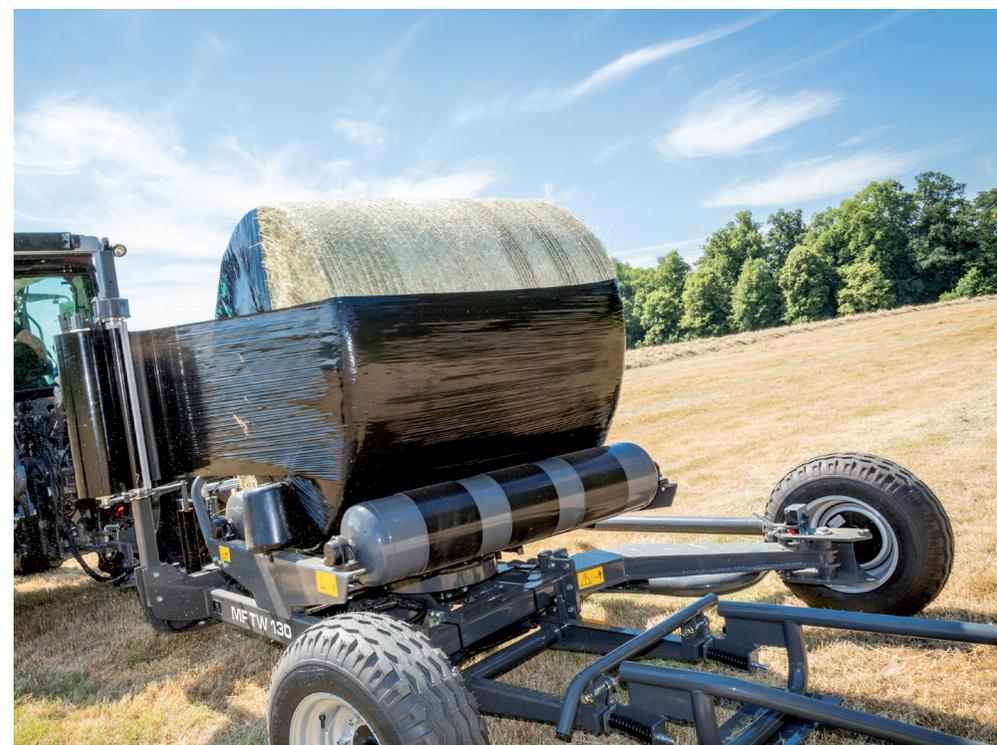
By simple adjustment, the right-hand side transport wheel can be turned around the centre spindle, extending the overall transport width from 2.50m to 2.85m, thus increasing the overall wrapper stability.
